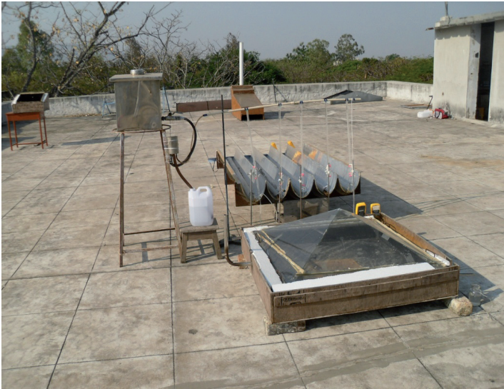
Figure 2. Pictorial view of compound parabolic concentrator tubular solar still coupled with pyramid solar still.
