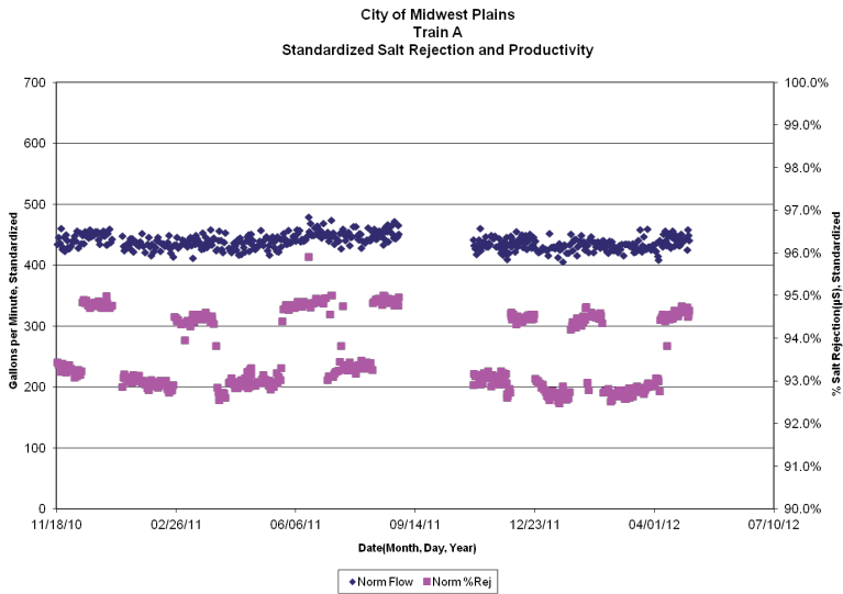
Figure 2. Standardized System Data: Permeate Productivity and Salt Rejection.
